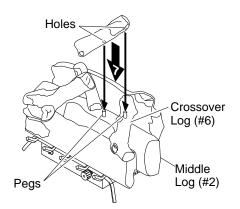
Figure 34 - Installing Crossover Log (#7) to Model CCL3930NTA Only
